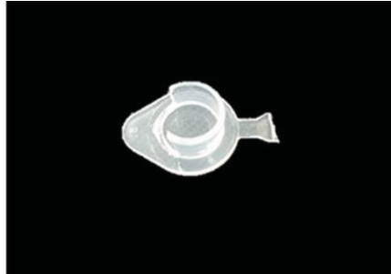
Supplementary Fig. S1. PCR tube lid with a manual cut. When moving embryos to PCR tube lids using glass micropipettes, the lid must be cut due to the shape of the glass micropipette.
